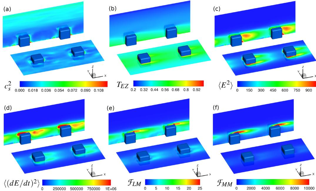
Figure 3: Contours across the domain of (a) the dynamic coefficient, (b) the dynamic time-scale in units of  $H/u_*$  where  $u_*$  is the friction velocity and  $H$  is the domain height, (c) mean square error in units of  $(u_*^4)^2$ , (d) the squared time derivative of the error in units of  $(u_*^5/H)^2$ , (e)  $\mathcal{F}_{LM}$  in units of  $u_*^4$ , and (f)  $\mathcal{F}_{MM}$  in units of  $u_*^4$ .
