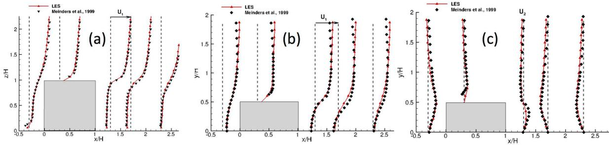
Figure 2: Mean velocity profiles predicted by LES using the dynamic time-scale (triangles) and experimental data from Ref. [5]. (a) Shows side view across center of cubes for streamwise mean velocity, (b) shows top view of half the domain, a cut through half the cube, streamwise and (c) transverse velocity.
