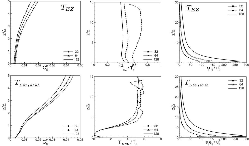
Figure 1: Left panels: profiles of dynamic coefficient. Middle panels: dynamically computed time-scale, scaled by the local reference turn-over time-scale  $T_\Delta = \Delta/u_\Delta = (\kappa z)/u_* \times (\Delta/\kappa z)^{2/3}$ . Right panels: average Germano-identity square error. Top panels use the dynamic time-scale  $T_{EZ} = 4\pi\tau_E$  while bottom panels use the traditional time-scale  $T_{LM,MM}$ .
